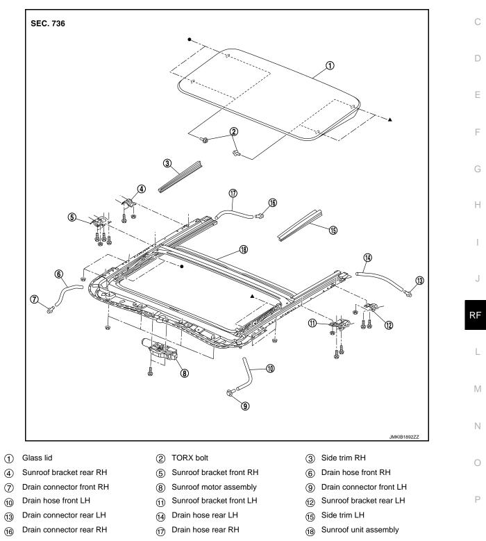
●,▲: Indicates that the part is connected at points with same symbol in actual vehicle.
